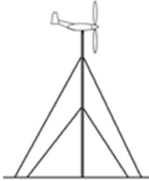
Figure[11]: Guyed Mast
